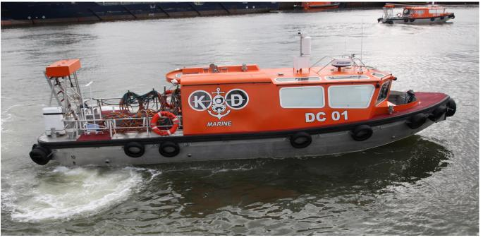
The KD Marine Daughter Craft DC01 and DC02 provide an enhanced and highly efficient access system for Divers or ROVs around offshore production installations and facilities. It also facilitates diving performed from non diving support vessels.
