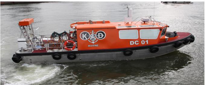
The KD Marine Daughter Craft DC01 and DC02 provide an enhanced and highly efficient access system for Divers or ROVs around offshore production installations and facilities. It also facilitates diving performed from non diving support vessels.
