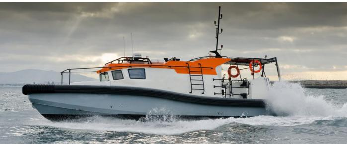
The KD Marine Daughter Craft provides an enhanced and highly efficient access system for Divers or ROVs around offshore production installations and facilities. They also facilitate diving to be performed from non-diving support vessels.
